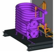
Double pipe heat exchanger
